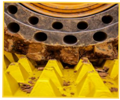
Pyramids effectively clean tires through compression and stretching without damage to the tire
